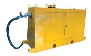
This system is designed for automatically reducing the alkalinity of waste water by dissolving Carbon Dioxide (CO2) into the flow to reduce the pH to between 7 and 10, making it safe for discharge.
