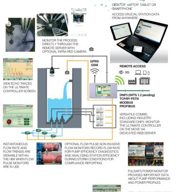
DETAILED PUMP INFORMATION AVAILABLE THROUGH THE HMI AND REMOTELY
