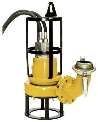
Discharge Size 150 mm Solids Size 65 mm Weight 140 kg Height 1100 mm Width (max.) 710 mm Max. Head 20 m Max. Output 94 l/s H.P. Nominal 20 kw Hvdraulic Flow 60 l/min Hydraulic Pressure 205 bar Power Pack 30 Series
