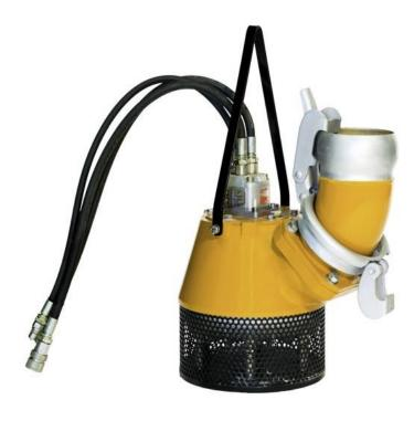
Discharge Size 150 mm Solids Size 10 mm Weight 55 kg Height 710 mm Width (max.) 560 mm Max. Head 31 m Max. Output 61 l/s H.P. Nominal 10 kw Hydraulic Flow 30 l/min Hydraulic Pressure 205 bar Power Pack 20 Series
