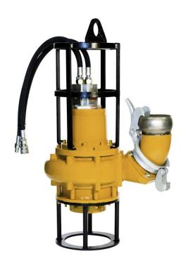
Discharge Size 150 mm Solids Size 100 mm Weight 250 kg Height 1153 mm Width (max.) 710 mm Max. Head 33 m Max. Output 99 l/s H.P. Nominal 20 kw Hvdraulic Flow 60 l/min Hydraulic Pressure 205 bar Power Pack 30 Series
